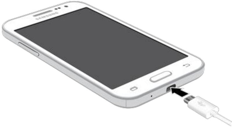
2. Insert the large end of the USB cable into a USB port on your computer.
